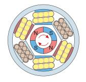
Brushless DC Motor with contact-free rotor eliminates wear and tear.
