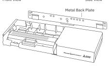
The Plasma Quad Connect slides into a metal fitment, which is screwed onto the back of the ducted unit.
