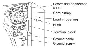
Operation requires a control switch. Have a control switch ready and connect the wiring shown in bold on the connection diagram below. Suitable cables: Ø0.5 to Ø2.0 mm diameter
