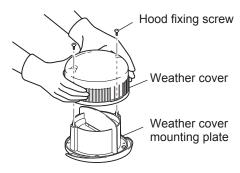
(2) Properly insert the groove section of the hood mounting plate to the partition of the air supply/exhaust pipe so that the "ウエ" mark comes to the top.
