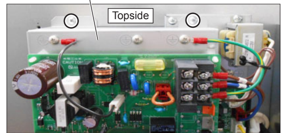
Base plate of PCB A
